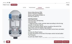
d) Diagnosis: with this function, the tire pressure system fault code can be read, the tire pressure system fault code can be cleared, the sensor ID number stored in the tire pressure system can be read, and the tire pressure function can be learned. (The diagnostic page may vary from vehicle to vehicle.)
