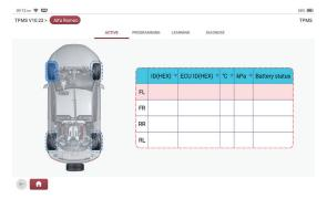
b) Programming: with this function, sensor data can be programmed to a blank THINKCAR sensor to replace one that is low on power and is not working properly. Three sensor programming methods are provided: automatic, manual and activation copy.
